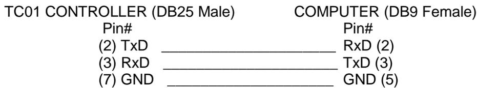
For TC01 Controllers with serial number C1508 or later, use the following settings to communicate through Windows:
