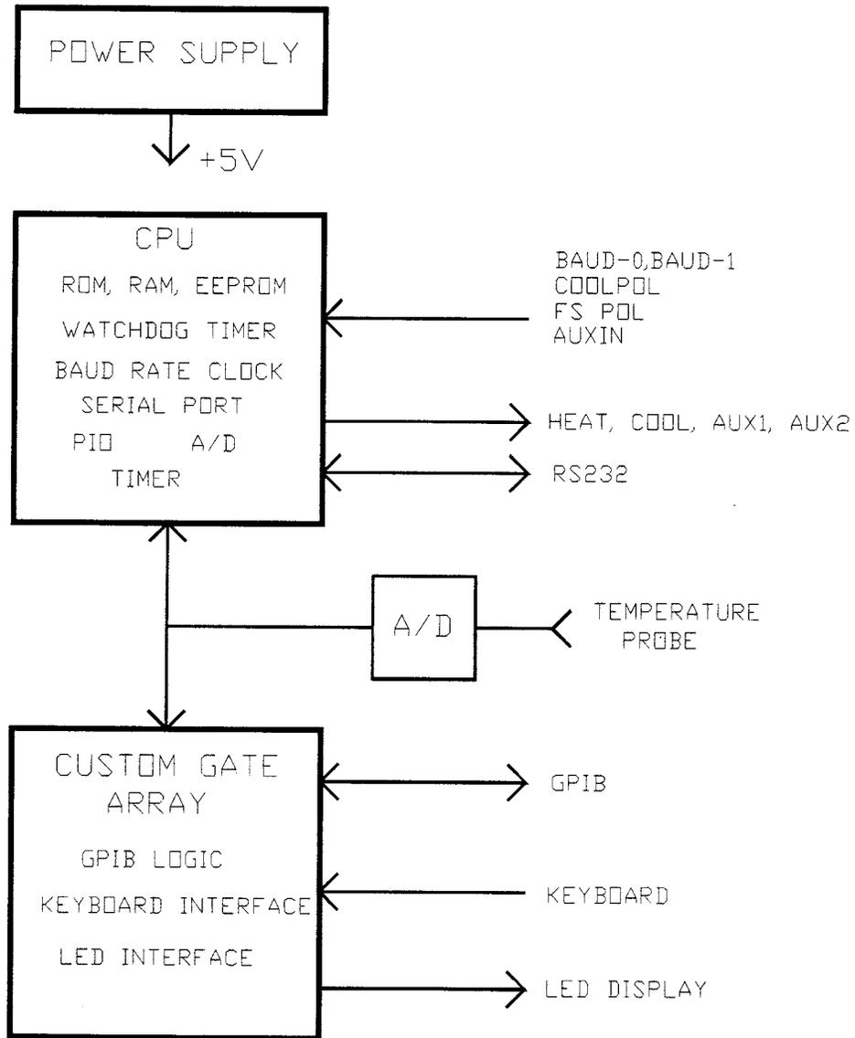
FIGURE 1 TC01 BLOCK DIAGRAM
